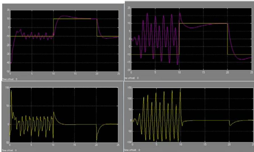
**Figure 9. Response of 2-DOF Helicopter. Pitch and Yaw angles and derivatives using frequency transition model.**
