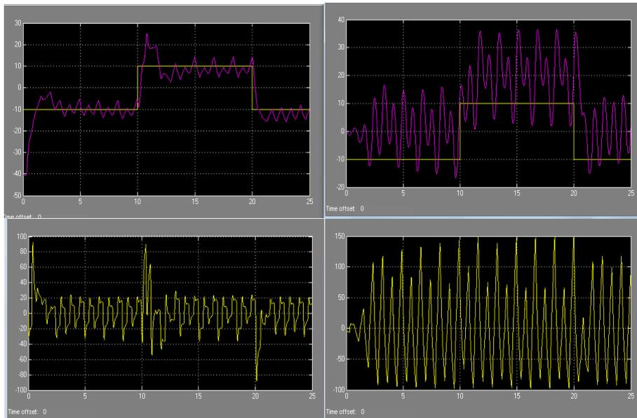
**Figure 8. Response of 2-DOF Helicopter. Pitch and Yaw angles and derivatives.**
