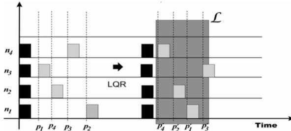
**Figure 2. Task periods controlled by LQR controller into a schedulable region.**
