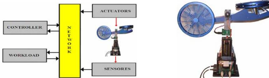
Figure 7. Networked Control System with workload.
