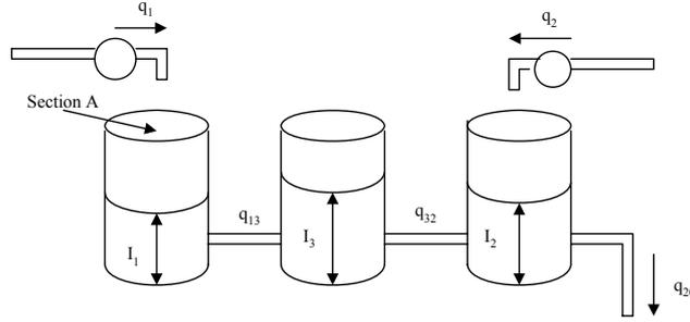
**Figure 3. Three tanks representation.**
